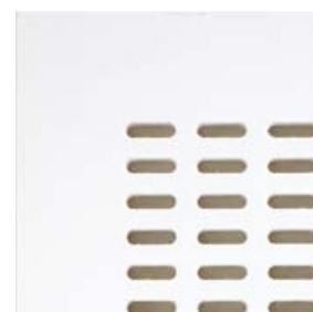
TANGENT 4 x 14 mm, 10/20 mm c/c Perforering: 13,3-15,0-15,8 %
