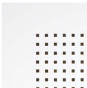
MICRO 3 x 3 mm, 8,3 mm c/c Perforering: 9,5-10,7 %
