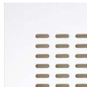
TANGENT 4 x 14 mm, 10/20 mm c/c Perforering: 21,6 %
