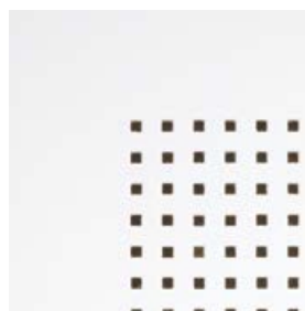
MICRO 3 x 3 mm, 8,3 mm c/c Perforering: 10,2 %
